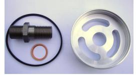
Remove the old seal which sits in the groove in the filter head. Replace with the new seal supplied in the kit. Place the alloy adaptor plate in position in the filter head and insert the hollow locating bolt (we recommend Loctite) and copper washer. Tighten the bolt using a 1" AF socket. You are now ready to fit a spin-on filter.
